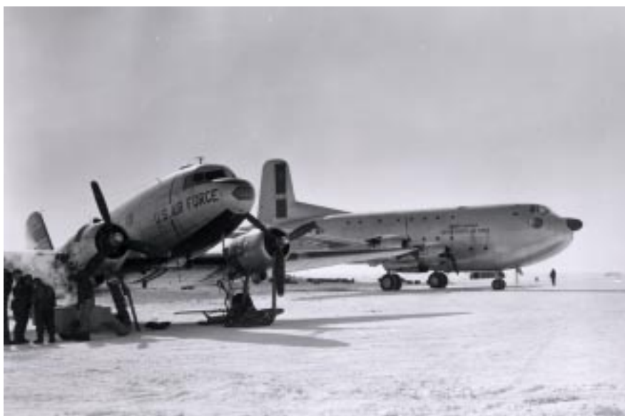
Lifeline. Isolated DEW Line sites were resupplied by aircraft such as the ski-equipped C-47 at left and the then-new C-124 at right. The flying was dangerous work; 25 people died in aircraft accidents in 1956 alone.
